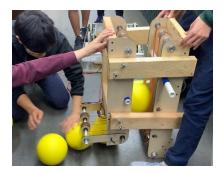
Horizontal Indexer: A wooden column with poly cord on pulleys used to test compression and slippage of balls.
