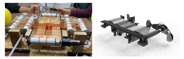
V-belts: We replaced the beavertail with v-belts, which allows us to intake and index multiple balls at the same time without jams.
