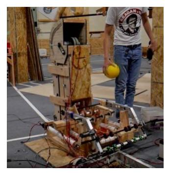
Integrated Prototype: The combination of four separate prototypes: the beavertail, horizontal indexer, intake, and shooter. It was used to test packaging and integration from the time the ball enters the robot, to the time it exits.
