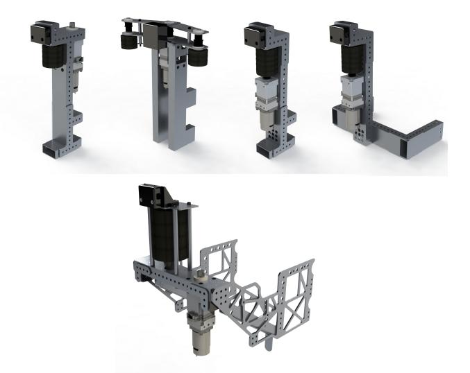
Our spinner mechanism went through 5 different iterations within CAD before being machined and physically tested. The final design contains multiple bent sheet metal parts to be able to withstand forces from all directions, as well as 3" flex wheels for reduced impact forces, and it is optimized to save weight and space.
